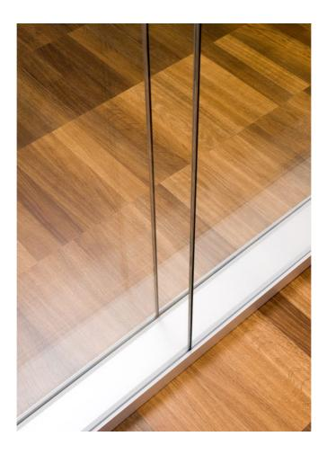
The construction consists of floor and ceiling-mounted profiles that support glazing elements (single-pane or laminated safety glass panes between 10 and 12 mm thick), where the edging uses a special acoustic cruciform joint. The wall thickness is 100 mm. The system can incorporate a variety of door types (solid, aluminium frame, fully glazed, flush-bonded glazing).
