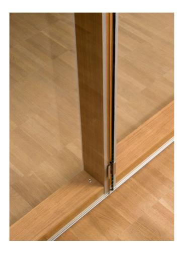
The supporting substructure consists of floor and ceiling-mounted profiles as well as mullions and transoms made from veneered wood products. The glazed elements on both sides are single-pane or laminated safety glass panes that are connected to the wooden mullions with clips. The wall thickness is 100 mm. The system can incorporate a variety of door types (solid, aluminium frame, fully glazed, flush-bonded glazing).
